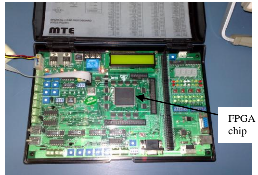
Fig.3 Photograph of Mechatronics make FPGA prototype board[12]
