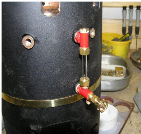
Figure 3 Water gauge fixed to boiler
