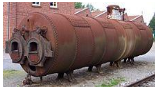
Figure 1 Industrial Boiler for supplying steam.
